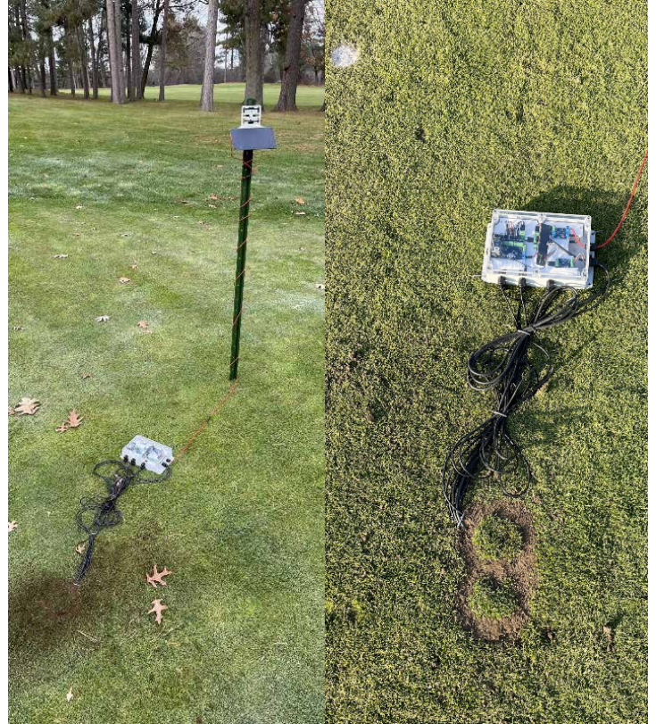
Figure 1. The winter sensors developed at the University of Minnesota. Solar-powered and cellular connected, these sensors will measure CO 2 and O 2 as well as temp and moisture levels at 3 different soil depths. You can track this data in real-time throughout the winter.
