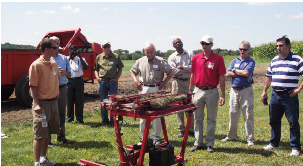
Shane and Doug demonstrate a research tool used to differentiate rooting strength between different sod samples
