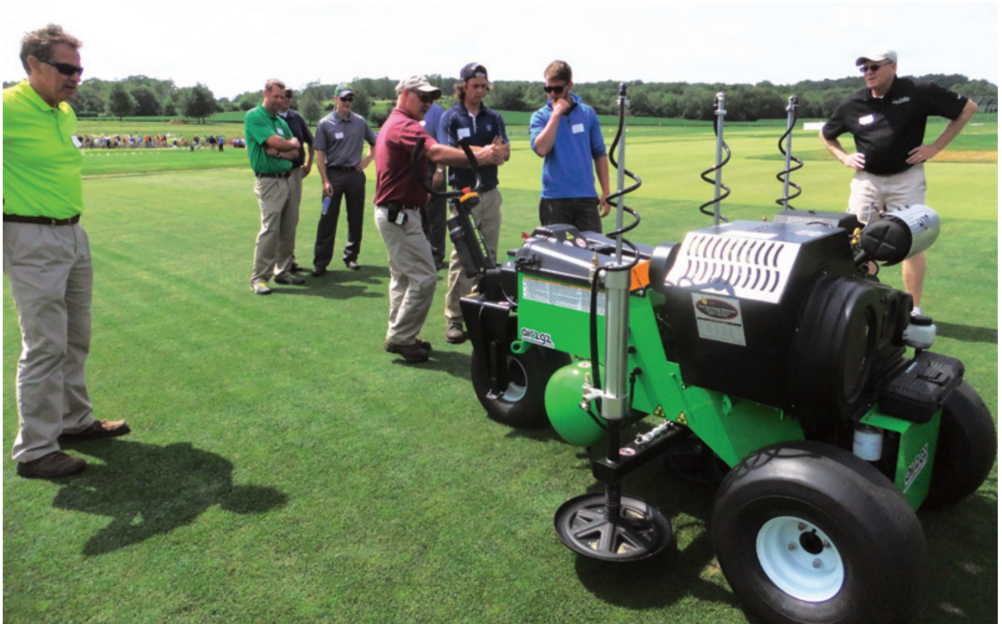
Representatives from Soil Solutions demonstrate their air injection machine to alleviate soil compaction
