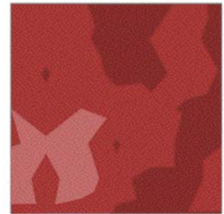
Figure 1: Adequate soil moisture uniformity from proper spacing of drip laterals.
